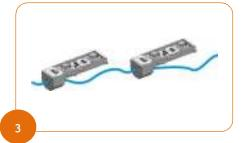
Use a 14 AWG stranded wire and thread all modules in series onto the wire.
